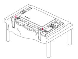
2 Use the screws to secure the stand on the rear side of the product as shown in the diagram.
